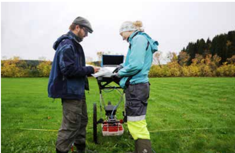
IMG. 04 — Archaeological geo-radar survey of the barrack's area at the Falstad Camp. Photo: Marek E. Jasinski.
